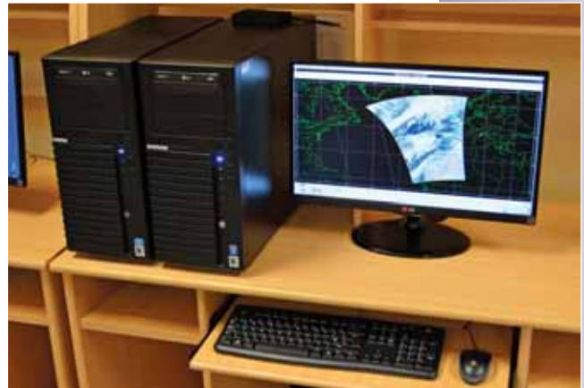
▲ Processor PC running RT-STPS, Simulcast, IPOPP and FY3L0pp/FY3L1pp software
