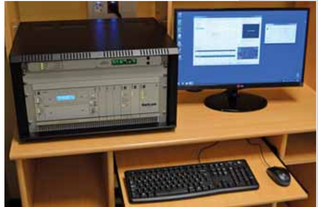
▲ Receiver rack, high-rate demodulator and ingest PC running 64-bit Windows with Dartcom Polar Orbiter Ingestor software
