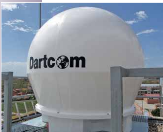
▲ Dartcom 1.5m X-Band antenna system at the University of Valladolid, Spain
