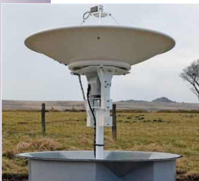
▲ Radome removed to show 1.5m parabolic dish antenna, scalar feed horn, LNA and BDC
